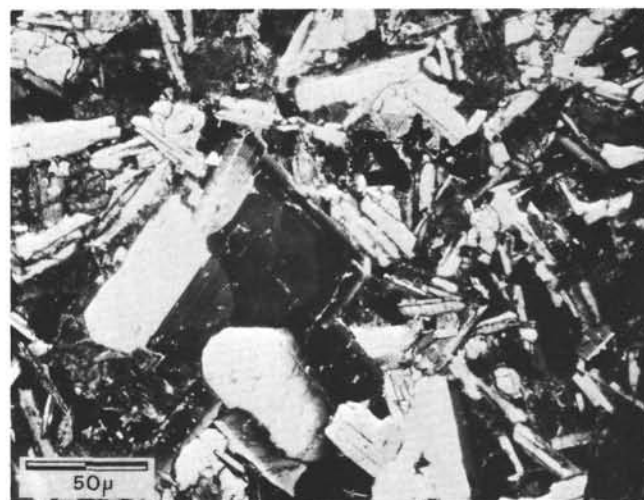
Figure 18. Sample DSDP 157-49-2(148), Carnegie Ridge. Glomeroporphyritic cluster of plagioclase showing euhedral oscillatory zoning and synneusis. Plagioclase is calcic labradorite with rims as sodic as andesine.
