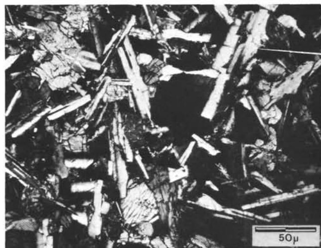
Figure 17. As shown Figure 16, but crossed nicols. Variable extinction shown by pyroxene in upper left corner is controlled by variations in composition, based on electron microprobe analysis.
